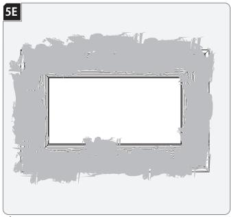
Properly plaster onto the plaster plate and drywall.
