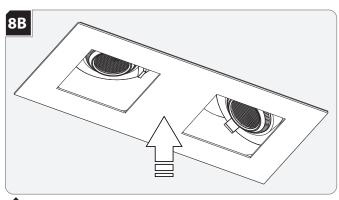
Gently push the trim into the lamp housing so all the brackets snap into place.
