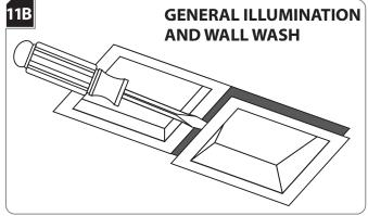
Remove the General Illumination and Wall Wash modules using a flathead screw driver to gently pry the module from the housing.
