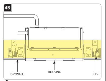
Align the cut out section of drywall with the housing and install drywall.
