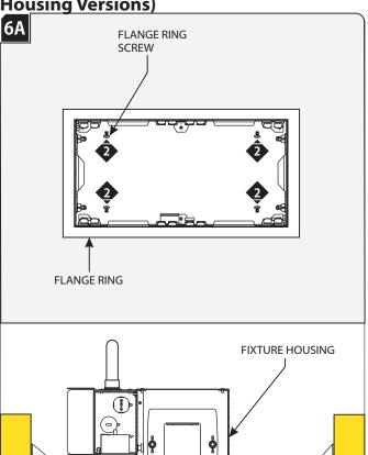
Insert the flange ring into the cut out and onto the fixture housing.
